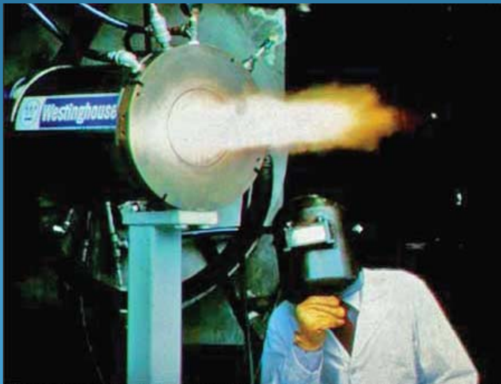
The plasma-heating unit creates the plasma arc used to turn trash into gas and rock-like material.
